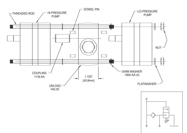
Current Endhead Design Uses 5/16-24 Mounting Thread. Older Endhead Design Used M8 Mounting Thread. Pump Kits Include Both Imperial And Metric Mounting Bolts.
