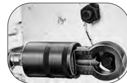
Align mark on cutter blade with scale.
