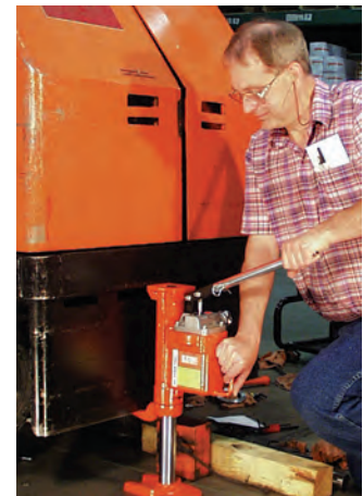
The J Series Toe Jack is an extremely rugged jack used here for lift truck service.
