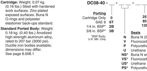
251.7 bar (25 psi) Standard855.9 bar (85 psi)1359.3 bar (135 psi)SealsNBuna N (Std.)VFluorocarbonPPolyurethaneUUrethaneNS\*Buna N with sealed spoolVS\*Fluorocarbon with sealed spoolUS\*Urethane with sealed spoolPS\*Polyurethane with sealed spool
